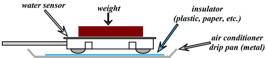
Note that the sensor depends on electrical conductivity to determine the presence of water underneath it. Therefore, distilled or deionized water may provoke little, if any response from the sensor, since such highly purified water is often only weakly conductive. Similarly, the sensor may not be suitable for detecting leaks of liquids other than water, if such liquids are not electrically conductive.
