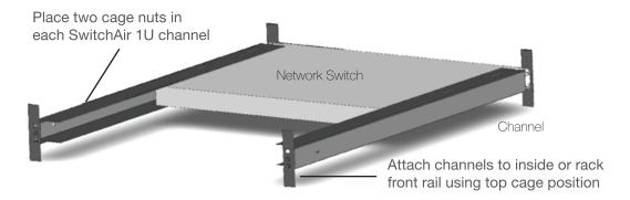
**STEP 2** Before installing SwitchAir; remove the lower network switch mounting screw from each side of the rack front rails. Save these screws to be used in the next step for mounting SwitchAir. The network switch upper screw will remain fastened. Attach Channels to Inside of Rack Front Rail Using Top Cage Position.
