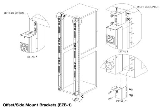
Using the offset/side mount brackets, attach PDU to rack as shown.
