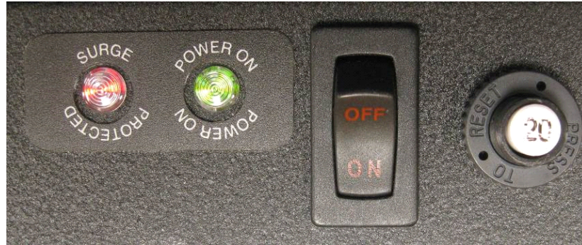
Figure 3-1 Surge Suppression LEDs
