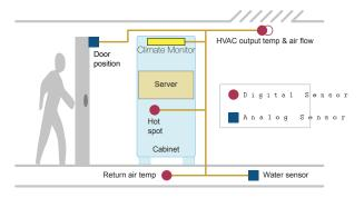
The server room uses a Watchdog 1200 to monitor the cabinet environment plus five external sensors to monitor thee A/C output, cabinet hotspots, return air temperature, water leaks and door position.
