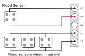
One or more flood sensors can be connected to each Analog Input or Analog to Digital Converter. Wired in parallel, a leak is detected if any of the sensors become wet.
