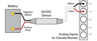
The pair of wires with ring terminals connect to a battery, while the other two signal wires attach to the Geist Climate Monitor.
