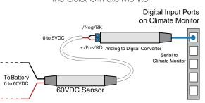
The Analog to Digital Converter acts as a bridge between the 60VDCM sensor and the digital sensor port.
