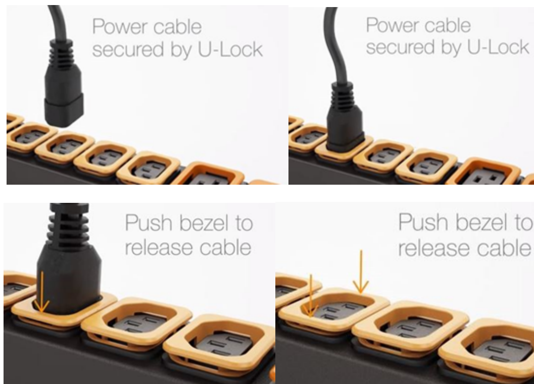
Figure 2-15 U-Lock Cord Retention Operation
