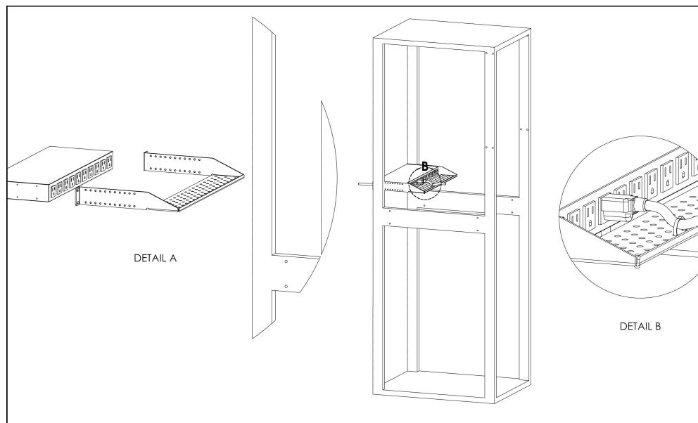
**19" Horizontal/Panel Mount Brackets (7938)**Figure 2-14 19" Horizontal/Panel Mount Brackets
