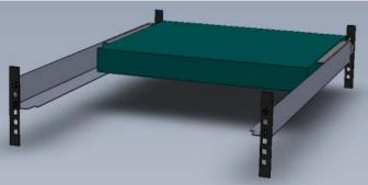
STEP 3: Before installing the chassis/extender the unit must be extended to the longest length. This is done by pulling the tabs on the chassis away from the extender. The cables that attach to the back of the data switch must be in place to route through the brush strips when the chassis/extender is pushed into place.
