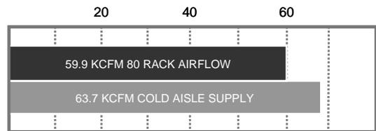
Total airflow consumption is compared to the total airflow supplied by looking at the AHU output volume. When AHU are speed controlled, airflow is directly proportional to fan speed.
