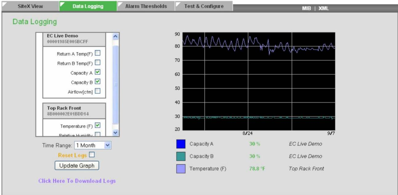
The vertical axis units scale adjusts based on the greatest units for a desired checkbox. To achieve greater visibility, select units with the same ranges before updating graph. Selecting checkboxes for viewing does not affect data logging. All data available is logged and kept for the past 1 month. The horizontal axis date scale adjusts based on the latest available data that data has been collected up to 1 month.
