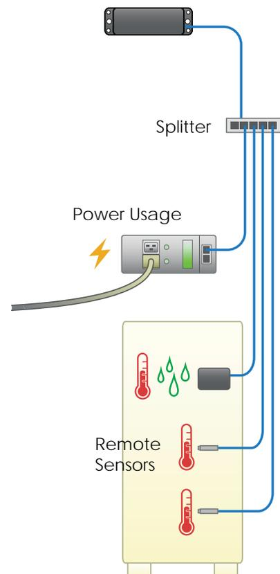
Using a splitter, the Watchdog 15-P supports up to four external sensors.
