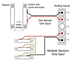
These sensors connect to the Geist Climate Monitor through the Analog Input terminals or Analog to Digital Converter. Sensors can be wired in series to reduce the number of inputs required.
