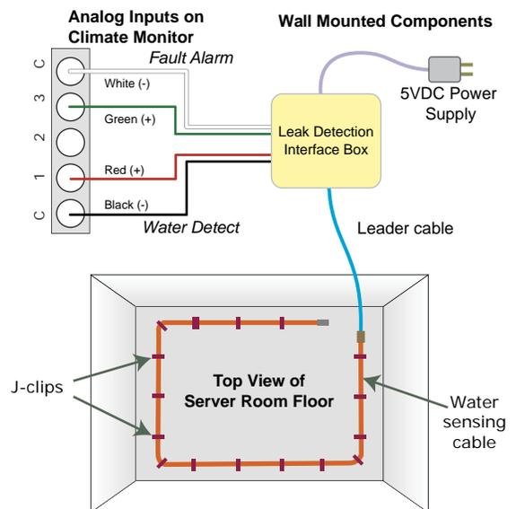
The sensing wire connects to the leader cable which goes to the interface box. Signals from the interface box run to the Geist Climate Monitor.
