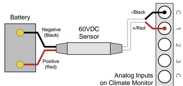
The pair of wires with ring terminals connect to a battery, while the other two signal wires attach to the Geist Climate Monitor.
