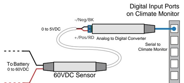
The Analog to Digital Converter acts as a bridge between the 60VDCM sensor and the digital sensor port.
