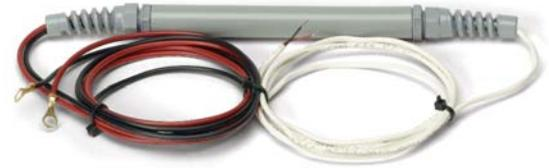
A plastic tube houses electronics that converts the 0-60VDC input voltage to a 0-5VDC signal compatible with the Geist Climate Monitor's analog input channels and protects against reversed polarity.
