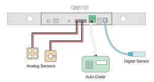
This diagram shows how remote sensors and an external device connect to the unit.
