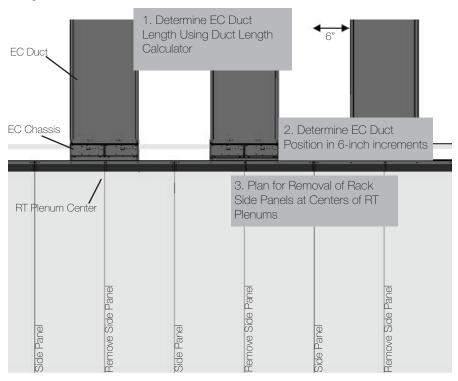
Variable positioning avoids over-rack obstructions such as cable trays and sprinkler heads, and allows you to add more managed heat containment capacity as needed.
