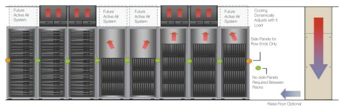
The 8-rack configuration shown is equipped with 4-systems for a total IT load capacity of 80 kW or 10 kW per rack average. Add systems as required for a total row load of 160 kW or 20kW per rack average.
