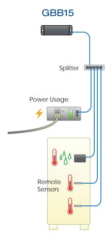
Using a splitter, the GBB15 supports up to 4 external sensors.
