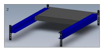
STEP 2 Slide the network switch into the rails and mount to the rack using customer provided cage nuts
