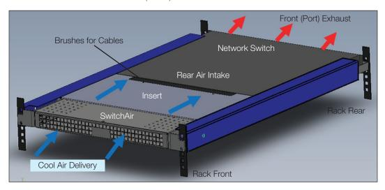
Delivers cool air to network switches with rear air intake and front (port) exhaust. Installs in minutes while network switch is live.
