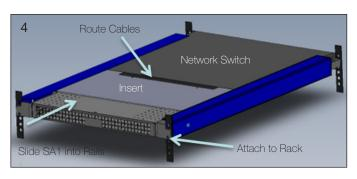
STEP 4 Insert SA1 into the rails and push unit until the insert comes into contact with the network switch and the chassis tabs are in contact with the rack. During this process route the cables through the brush openings. Install the bottom SA1 chassis screws on both sides.
