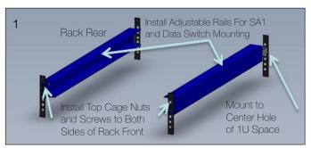
STEP 1 Mount the adjustable rails using customer provided cage nuts and screws. The new build rails will be used to support the network switch, SwitchAir chassis and insert. Attach the new rails using only the top front screw holes on both rack front rails. The rail extension tab attaches to the rack rear using a single cage nut and screw. Use the center hold of the 1U space for this attachment.
