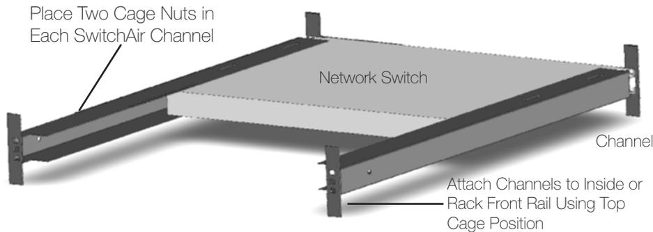
**STEP 2** Before installing SwitchAir; remove the lower network switch mounting screw from each side of the rack front rails. Save these screws to be used in the next step for mounting SwitchAir. The network switch upper screw will remain fastened. Attach Channels to Inside of Rack Front Rail Using Top Cage Position.
