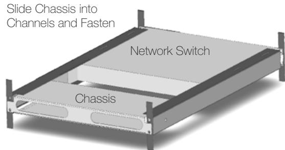
**STEP 3** SwitchAir is in a fully extended position when shipped from the factory. Insert SwitchAir into the open rack space at the same U height as the switch. As SwitchAir is pushed into the space, the SwitchAir Rail Tabs will engage the network switch rails for support during installation. Keep pushing the SwitchAir into the space until the SwitchAir front mounting flanges are flush with the rack front rails. Reinstall the screws that were removed previously. Installation is now complete.
