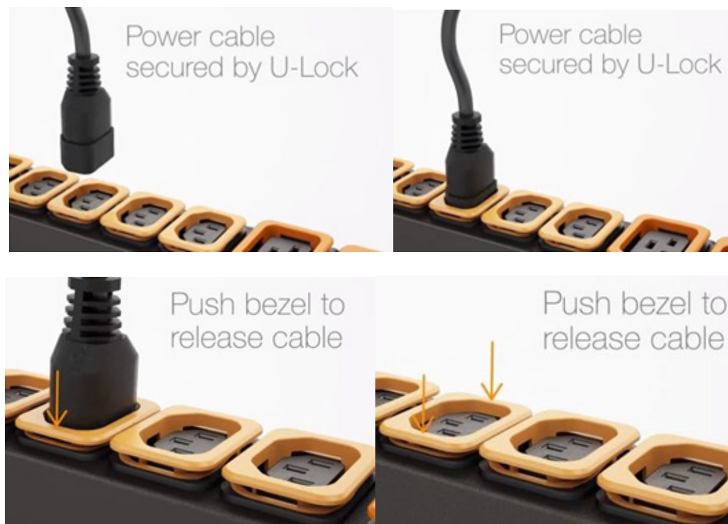
Figure 2-15 U-Lock Cord Retention Operation
