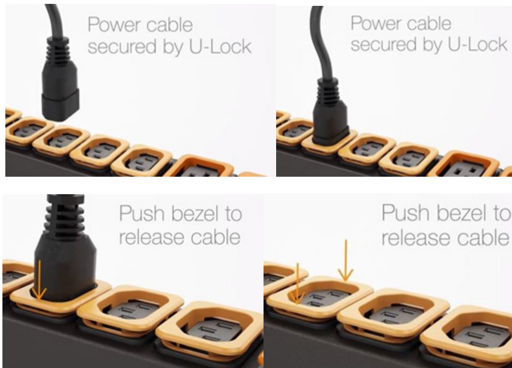
Figure 2-15 U-Lock Cord Retention Operation
