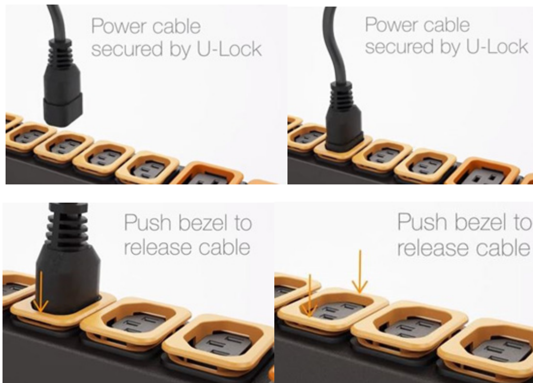
Figure 2-15 U-Lock Cord Retention Operation
