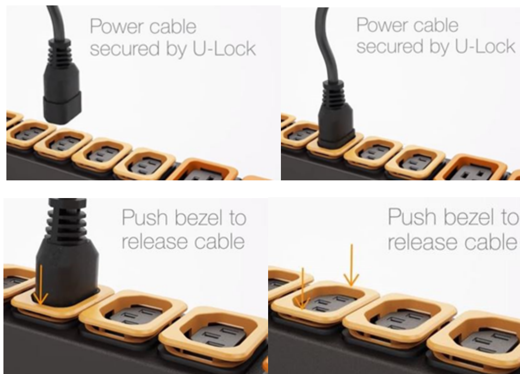
Figure 2-15 U-Lock Cord Retention Operation
