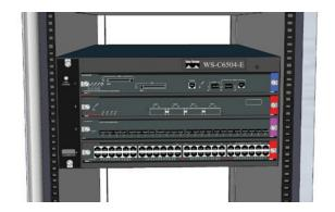
(2) Install support rail and air channel above or below device in the 2 RU of dedicated rack space.
